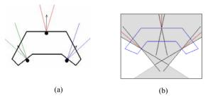
Figure 9: a) no force-closure 2D grasp, b) central axes of grasp wrenches ( $\alpha = 10^{\circ}$ ).Grasp wrenches can't exert a force along ( $-\mathbf{Y}$ ) axis and can't generate torques in two-direction in unreachable zones in (b).
