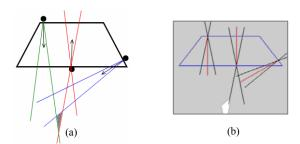
Figure 8: a) no force-closure 2D grasp, b) central axes of grasp wrenches ( $\alpha = 10^{\circ}$ ). Grasp wrenches can't generate a negative torque in grey zone.
