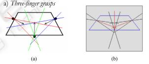
Figure 6: a) a three-finger force-closure 2D grasp, b) central axes of grasp wrenches ( $\alpha = 15^{\circ}$ ).
