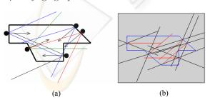
Figure 11: a) five-finger force-closure 2D grasp, b) central axes of grasp wrenches ( $\alpha = 25^{\circ}$ ).
