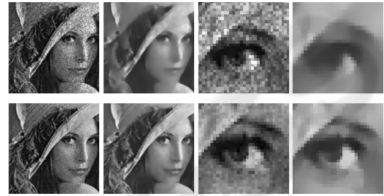
Figure 8: \frac{a|b|c|d}{e|f|g|h} . Image denoising using the suggested method. (a)(b) Speckle noise image and denoising. (c)(d) Zoom in from (a)(b) respectively, 100 iterations. (e)(f) Poisson noise image and denoising. (g)(h) Zoom in from (e)(f) respectively, 100 iteration.
