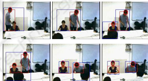
Figure 13: Tracking results before starting of the meeting, in which head pose estimation and hand tracking are not performed.
