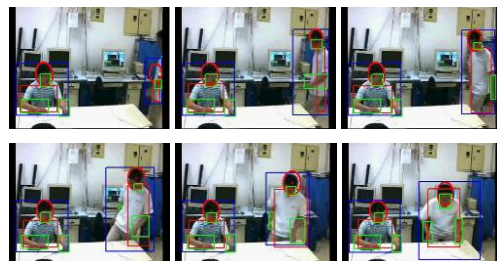
Figure 14: Human verification and tracking results while the presenter is walking back to his seat and sitting down.
