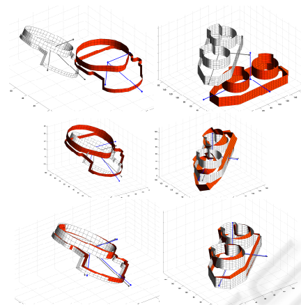
Figure 6: Pre-alignment comparison of PCA and 2D alignment. Initial position (upper row), PCA pre-alignment result (middle row) and computed pose after the first iteration of the correlation-based ICP (lower row).
