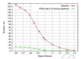
Figure 7: The EFSAT implementation is integrated into a hierarchical collision detection accelerator hardware. The overall design still yields a speed-up of an order of magnitude compared to a state-of-the-art software implementation. The latter does not provide categorization of exact results or any guarantees on correctness.
