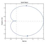
Figure 3: Nyquist plot of a transfer function G.
