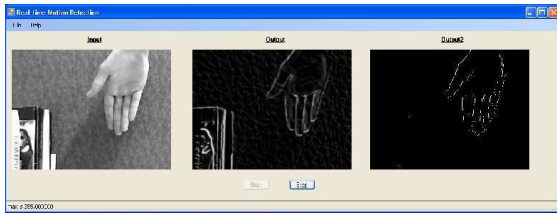
Figure 5: Real-time implementation. A code templates are displayed in the output. Only the hand is moving to the right direction. left: input image, middle: filtered image, right: output of the motion detector.
