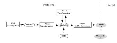
Fig. 2. Generator front-end.
