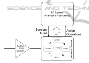
Figure 1: Autonomic Computing Model for ED.
