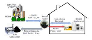
Figure 1: Simplified diagram of the operating environment of smart appliances in the context of smart grids.
