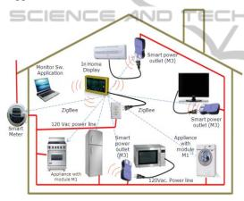
Figure 5: ZigBee communications network.
