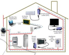
Figure 6: PLC communications network.
