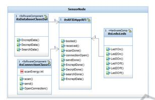
Figure 2: RFID Class Diagram.
