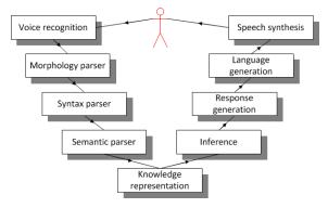
Figure 1: Concept of a dialog system (Schneider, 2012).
