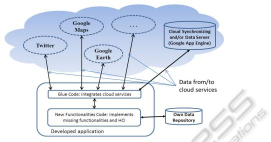
Figure 2: The picture shows the logical general schema of the proposed architecture.
