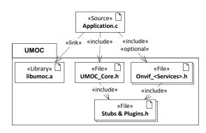
Figure 2: UMOC structure and usage.
