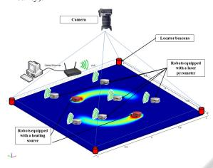
Figure 2: Representation of the experimental prototype.
