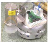
Figure 3: Khepera robot equipped with a Laser pyrometer.
