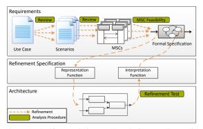
Figure 2: Artifacts, relations and analysis procedures with focus on functional requirements and their mapping onto the architecture.
