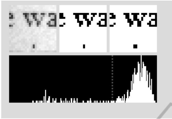
Figure 3: The upper left panel shows a noisy tile, whereas the upper right panel shows the noise-free (ground truth) tile. The upper middle panel shows the binarized version of the noisy tile, using the optimal binarization threshold indicated by a vertical dotted line in the histogram (lower panel).
