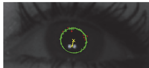
Figure 2: Eye tracking features extracted from each eye. Blue: Corneal reflections. Yellow: PCCR vector. Green and red: Edge points found by the starburst algorithm (Red points were rejected by RANSAC step).
