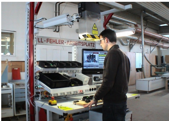
Figure 1: Smart assembly work place with assistance display (DESC leanworkStation).
