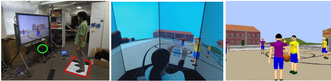
Figure 2: Virtual basketball (left) being played through the use of a Kinect sensor and a foot pressure pad. These sensors are combined and used in the immersive display setup (center). The right image shows a screenshot of the game.
