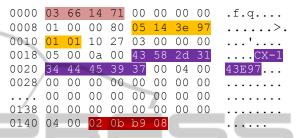
Figure 2: Information sent from the PLC to the EWS as reply to a search request.
