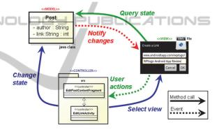
Figure 1: MVC structure of the WordPress app.
