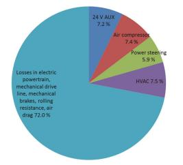
Figure 4: Measured share of auxiliary component energy consumption in electric city bus during real-life operation on Line 11 in Espoo, Finland at 15 °C ambient temperature.
