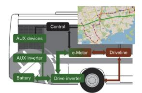
Figure 5: Subsystems of the auxiliary device energy consumption model. The coordinate data is included in the model, shown in a map at the top of the figure.
