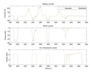
Figure 7: Simulated battery current, motor power and air compressor power for baseline and optimal air compressor operation during part of the cycle length.
