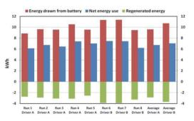
Figure 2: In-service electric energy consumption of a test bus running on Line 11, in city of Espoo.
