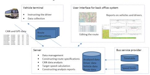
Figure 3: Communication between the components of the driver assistance system.
