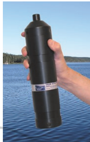
Figure 3: VR2W acoustic receiver.
