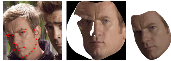
Figure 9: An example result of the landmark fitting. (left): Input image from LFPW. (middle): The extracted face texture as isomap. Regions of self-occlusion are depicted in white. (right): Resulting shape and camera model fitting.
