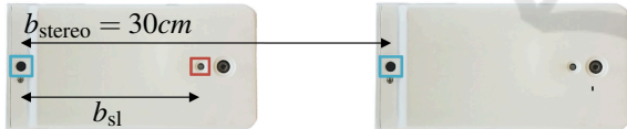
Figure 2: Recording depth images with the Project Tango device: The smartphone is moved by b_{stereo} to capture a stereo image pair. Simultaneously, the internal SL chip computes a depth image using the projected IR pattern which has an effective baseline of b_{sl} , which we determined in a calibration process.
