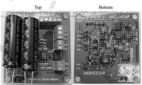
Figure 2: Developed energy harvester prototype.
