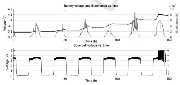
Figure 5: Energy harvester performance over six days.
