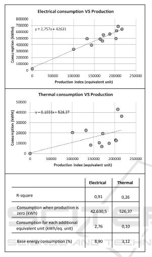
Figure 4: One of ESET Tool outputs (regression analysis) from a real case. The electric consumption shows a strong relationship with the production, while the thermal consumption appears poorly related (due to winter heating, production changes, other).
