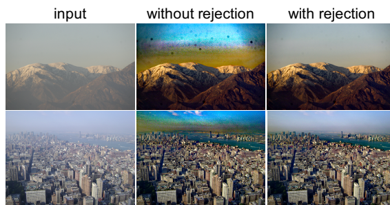
Figure 11: Validation of our narrow angle outlier rejection method described in Section 3. In the second column, the distant region represented as sky has an infinite depth, and hence our transmission estimation stage estimates its transmission as being close to zero, which yields overly saturated results. We obtained consistent results by our outlier rejection stage, as shown in the third column.
