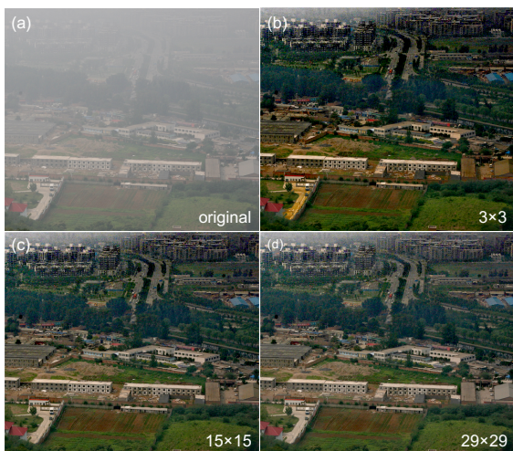
Figure 10: Comparisons to show the influence of a patch size in estimating transmission. (a) The original canon image. (b) The dehazed image with a patch size of 3 \times 3 where severe color clamping happens. (c) The dehazed image with a patch size of 15 \times 15 , which is our choice for all results. (d) The dehazed image with a patch size of 29 \times 29 in which the airlight in distant regions is underestimated.
