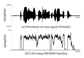
Figure 5: Comparison among VAD methods in sentence (female) (a) voice signal (b) fundamental frequency (c) VAD using SHODEO function.
