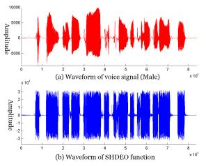
Figure 1: (a) Waveform of voice signal (Male) (b) Waveform of SHODEO function.
