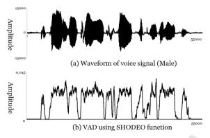
Figure 3: Comparison among VAD methods in word (male) (a) waveform of voice signal (b) VAD using SHODEO function.
