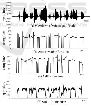
Figure 2: Comparison among VAD methods in sentence (a) waveform of voice signal (b) ACF (c) AMDF (d) SHODEO.
