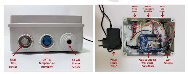
Figure 2: Smart Device Prototype Implementation.
