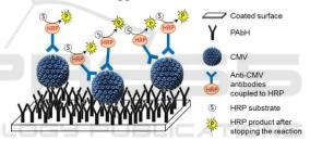
Figure 1: Principle of the HCMV biosensor.
