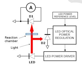
Figure 4: Schematic representation of the driving and detection electronics.
