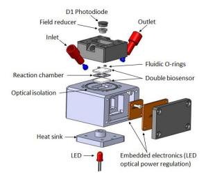
Figure 3: CAD view of the new opto-fluidic prototype.
