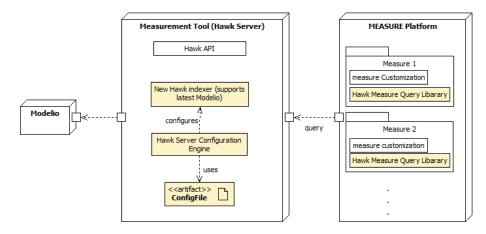
Figure 5: UML deployment diagram of the integration between Hawk and the MEASURE platform.
