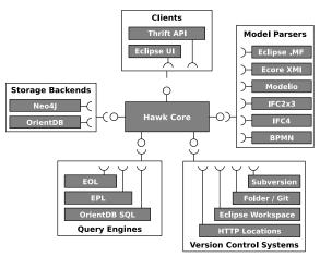
Figure 4: Component-based architecture of the Hawk model indexing framework.
