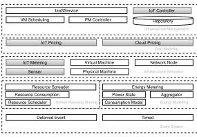
Figure 1: The architecture of the DISSECT-CF simulator .
