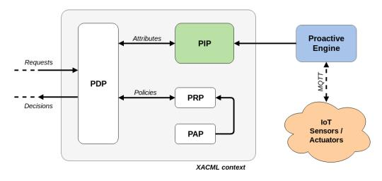
Figure 1: Enhanced ABAC model architecture.
