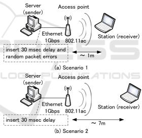
Figure 6: Experimental configuration.
