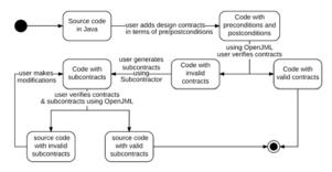
Figure 1: State diagram of the programming code in Subcontractor.
