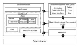
Figure 3: Subcontractor in Eclipse architecture.
