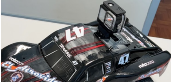
Figure 2: Assembly of the prototype for the remote-controlled vehicle used in the data acquisition process.
