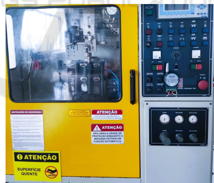
Figure 1: An industrial retrofit: machine with an adapted IIoT device. A common case in the Industrial environment.
