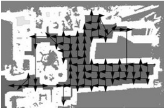
Figure 5: Waypoint generated for complete network test coverage.
