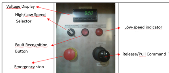
Figure 9: Hydraulic Pump Control Panel.
