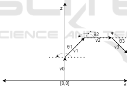
Figure 2: Two-Dimensional Vector Representation of Arm Configuration.
