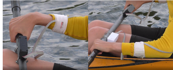
Figure 3: Strain gauges attached to the athlete's paddle.
