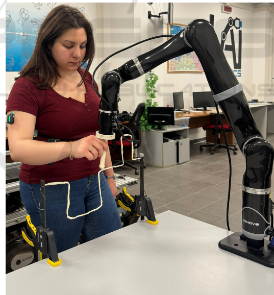
Figure 1: The scenario shows the experimental setup in which a human operator performs a co-manipulation task wearing four EMG sensors and using a Jaco 2 manipulator.
