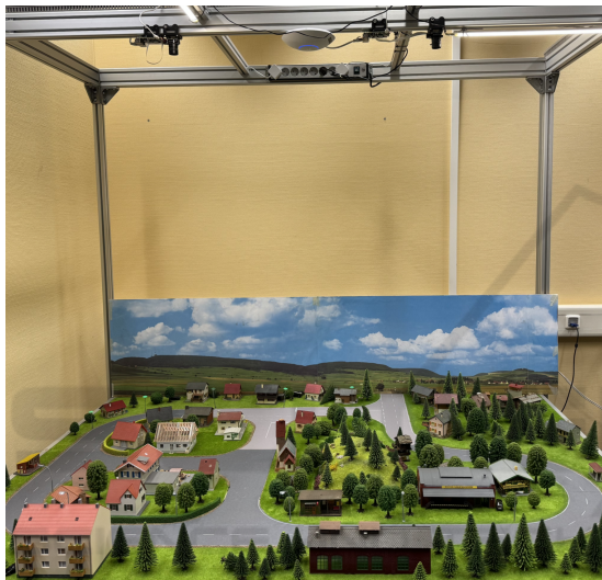
Figure 2: The figure shows the model world with streets, a hill in the centre, houses and a rural background image. At the top two cameras can be seen, each connected to an RPi, and lamps.
