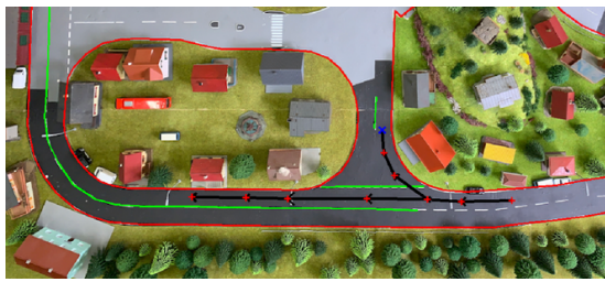
Figure 1: Excerpt from the model landscape for testing autonomous vehicles. The realistic complexity of the model with different road colours, road markings, trees, buildings, etc. can be seen. The functionality of the Mapbuilder tool, which is used to generate a precise simulation of the real test environment, is also visualised.
