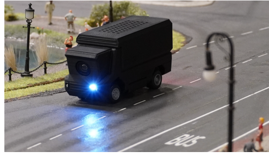
Figure 4: Tincar shown in Miniature Wonderland in Hamburg. The front facing camera is integrated into the windshield. A single LED is used as a headlight. The Tincar is also equipped with blinkers on each side.
