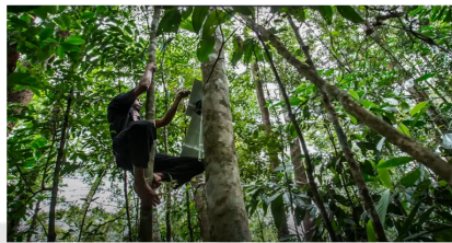
Figure 9: Team member Sacha, next to a mobile device, equipped with an audio sensor, an old smartphone.
