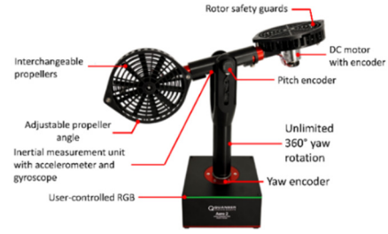
Figure 1: Quanser Aero2 helicopter system (Quanser, 2022a).
