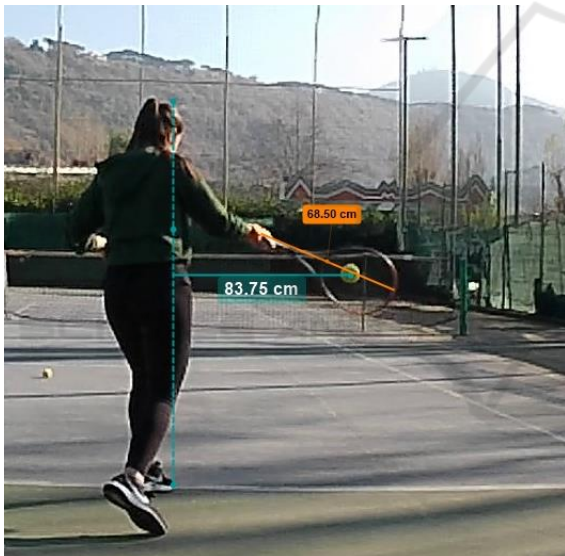
Figure 1: Distance measurement by video analysis. The racket measurement was used as a reference placed on the measurement plane in the calibration process.
