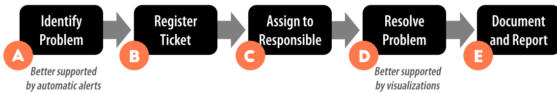
Figure 6: Facility management workflow derived from interviews. After identifying a problem (A), a ticket is created manually or by email (B). Such tickets represent a new entry on the backlog, which is classified and assigned to a responsible person (C). This person will then understand and resolve the problem (D). Finally, the process and results are documented and reported (E). Results show that although the visualization dashboards were created to support identifying problems (A), they were actually mentioned to better support understanding and locating the problem (D).
