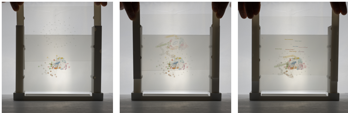
Figure 4: Composition of a HoloGraph . Focus slices show the nodes of interest at every timeslice. Context slices can be added to each focus slice individually (a). Node trajectories of focus nodes can be added as a global overlay (b), together with focus node labels (c).
